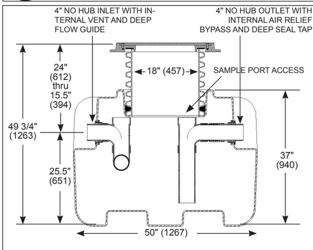
\*Note: The FE 750 does not meet PDI standard if outfitted with an internal flow control (-OP suffix). The PDI standard is only valid for the external flow control fitting.
